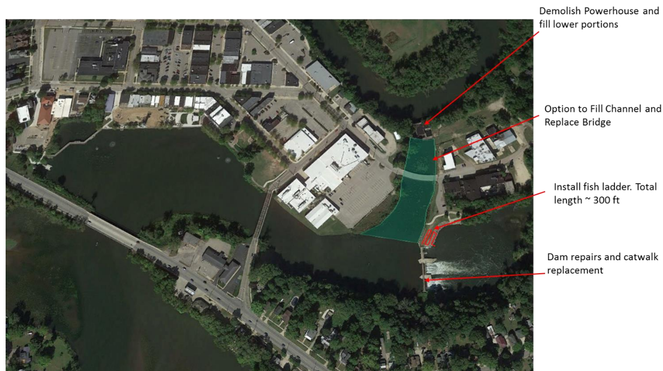
Figure 10. Site Overview for Dam Repair/Maintenance Alternative.
